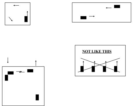
MISTRAAL FANS ARE DESIGNED TO MEET THE REQUIRMENTS OF THE EUROPEAN COMMUNITY MACHINERY DIRECTIVE. FOR THE INSTALLATION TO MEET THESE REQUIREMENTS WE RECOMMEND THE FAN BE INSTALLED AT A MINIMUM HEIGHT OF 2.4mts FROM THE FLOOR.
